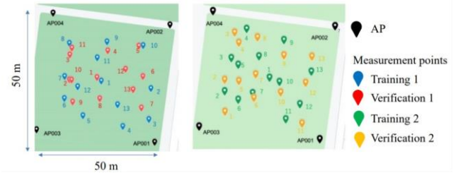
Fig. 6 – Measurement setup and location of the first dataset
